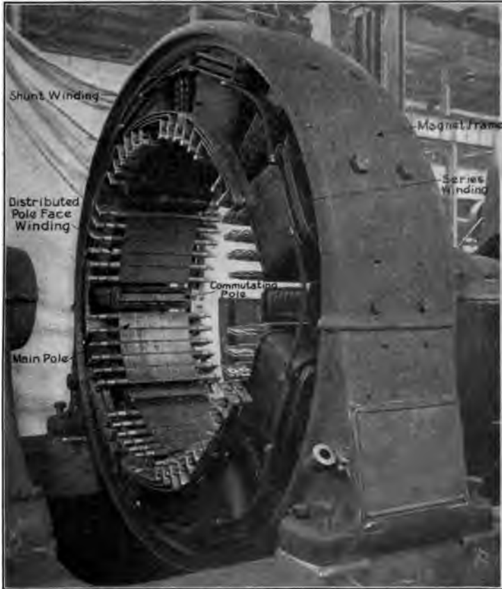
FIG. 16.—Field construction of compound wound generator with commutating poles and compensating windings.
